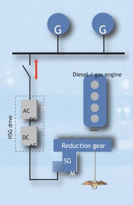
In current hybrid systems (shown left) power generating requires a fixed engine rpm when operating the shaft generator, and does not allow the shaft generator to operate in parallel with the auxiliary gen sets.
