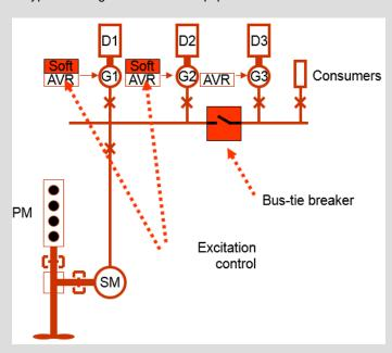
As with the Auto-Transformer Start described in Option 2, the machine is started asynchronously and so requires some excitation system modifications.
