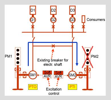
With two identical shaft generators, it is possible to swap over the PTO and PTI/PTH modes of operation from one side to the other.
